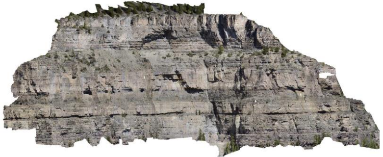
Hanging Lake Slope, Colorado, USA. Monitoring of a rock wall affected by rock falls: 550 m high, 900 m wide with a precision of 12 mm, and a 10-mm pixel size on the rock slope.
